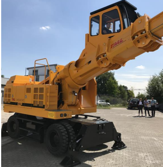
UNIDACHS 640P with tiltable driver's cabin
